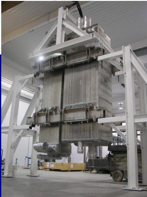
Internal Heat Exchangers
